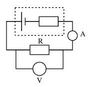
R A in series 1 R (can be variable) 1 A and V correct V as shown
