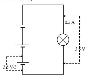
Voltage across each circuit component and current in lamp: Either 3.5 V/3 shown across the terminals of one cell or 3.5 V across all three cells 3.5 V shown to be across the lamp 0.3 A flowing in the lamp [i.e. an isolated 0.3 A near the lamp does not score]
